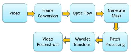
Fig 1: - block diagram of proposed system
